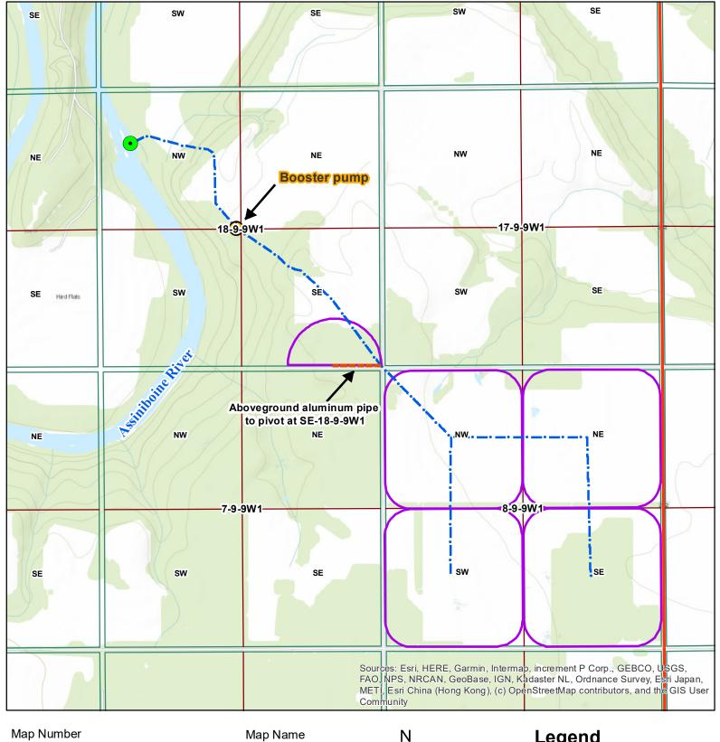
Legend **Project Infrastructure** 3 rev Intake Pump **Project Name Booster Pump** 125 250 750 1,000 Swansfleet Irrigation Project Pipeline Meters **Pivot** PREPARED BY DRAWING SCALE DATE DRAWN/CHECKED 1:20,000 November 20, 2023 DAW/PBS Provincial roads
